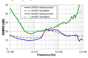
Fig. 11. Comparison between measurement and simulation of the EMIRR of the LMV651 and LMV861
