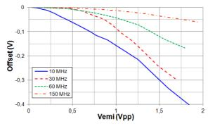
Fig. 8. Evolution of the offset measured on LMV861 (EMI-hardened) output vs. EM disturbance amplitude and frequency
