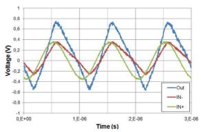
Fig. 7. Illustration of slew rate asymmetry: injection of a 1 MHz continuous wave disturbance on non-inverting input of LMV651  $\,$
