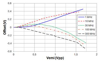
Fig. 6. Evolution of the offset measured on LMV651 (non EMI-hardened) output vs. EM disturbance amplitude and frequency
