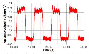
Fig. 3. Illustration of non-linear behavior of op-amp to EM disturbance: output signal measured on LMV651 when a 500 MHz amplitude-modulated perturbation is added is coupled on the non-inverting terminal
