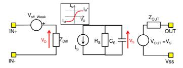
Fig. 10. Structure of the general analog behavioral model of op-amp
