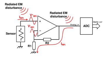
Fig. 1. Typical scenario of coupling EM disturbance on conditioning signal stage
