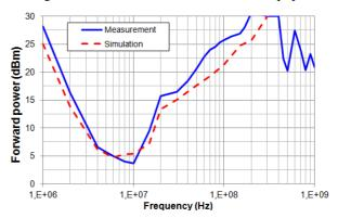
Fig. 13. Comparison between measurement and simulation of the susceptibility level of the LMV651 in another configuration (follower and external low-pass filter)
